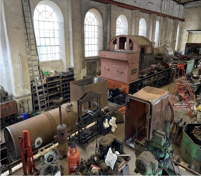
Since our last update, work has continued on the inner firebox of 563. This has included the team marking and drilling out countless holes in the inner firebox for the stays.
