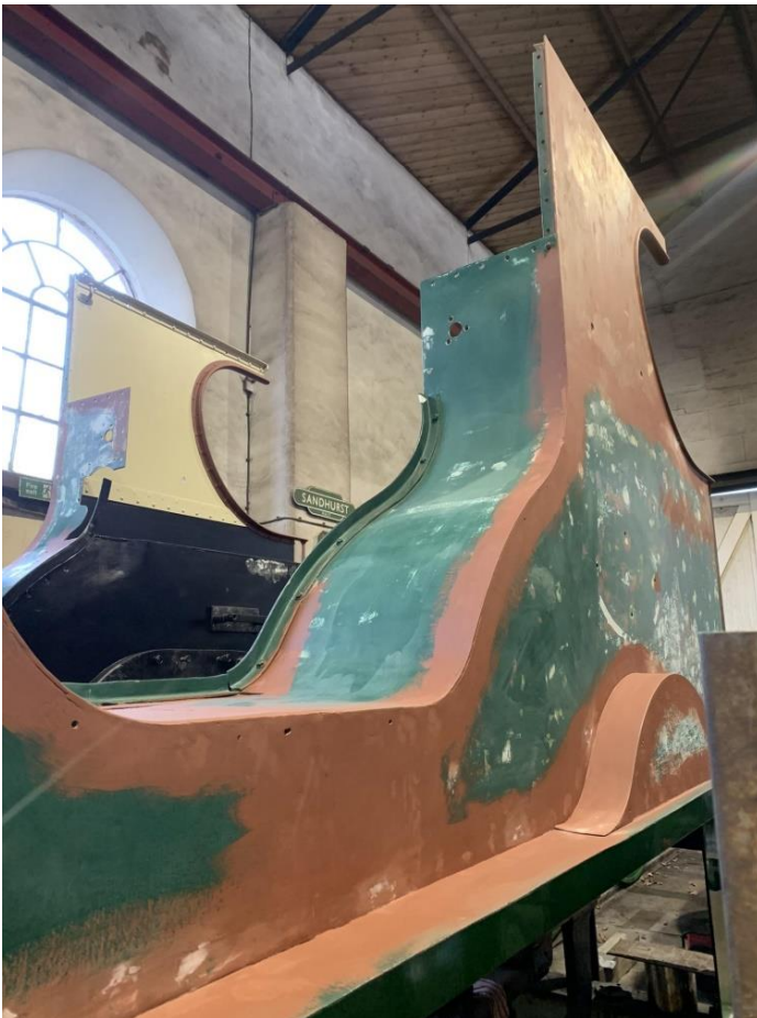
Work continues on preparing the cab sides and splashers for further coats of paint and test fitting the brass beading.
