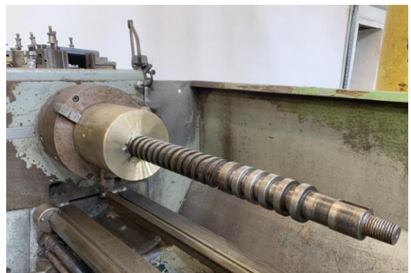
The start of a new nut for the reverser can be seen at the far end, ready for squaring off.
