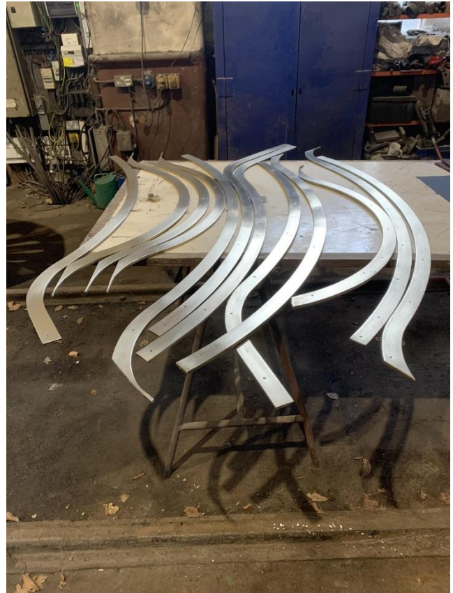
The brass beading being cleaned up ready for trial fitment on the splashers.
