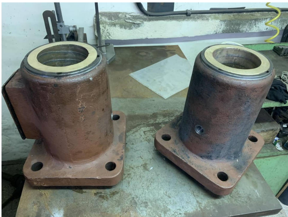
The machined cannon boxes with new bronze liners that guide the valve rods.
