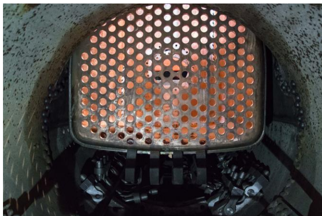
The view from within the upside down boiler barrel. The girder and sling stays can be seen at the bottom and once fixed in place, these will support the inner firebox assembly.
