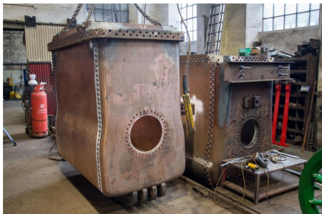
The inner firebox (left) prior to final test fit where it'll be lowered into the outer firebox (right).
