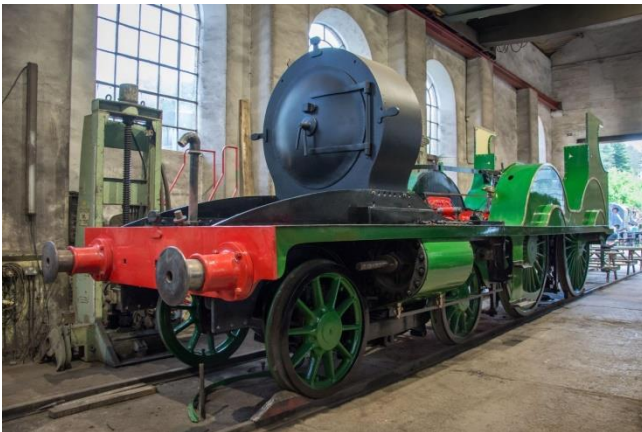
563 now re-wheeled and awaiting the boiler to be finished.
