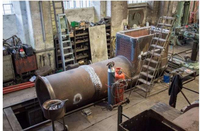
563's upturned boiler with the inner firebox now installed.
