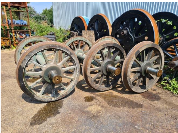
The tender wheelsets passed the ultrasonic testing so thankfully there are no cracks!
