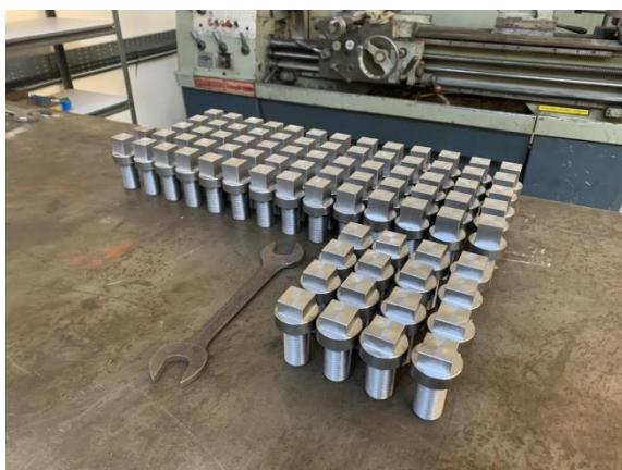
Newly machined crown stay bolts ready for fitting.
