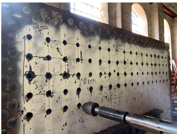
Holes for the stays being drilled, viewed from the outer firebox.
