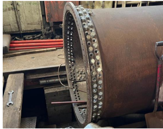
The angle ring at the front of the boiler has temporarily been bolted to hold it place, before riveting.
