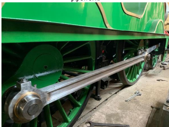
Connecting and con rods have been refitted.
