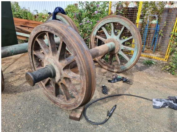
The tender wheelsets now need needle gunning before the axles go for polishing.
