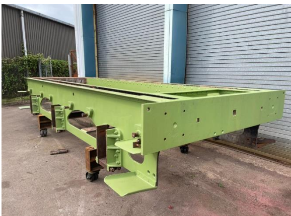
The tender frames after priming.
