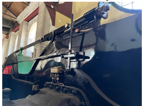
The lubrication pipework and trays have been fitted in the cab.
