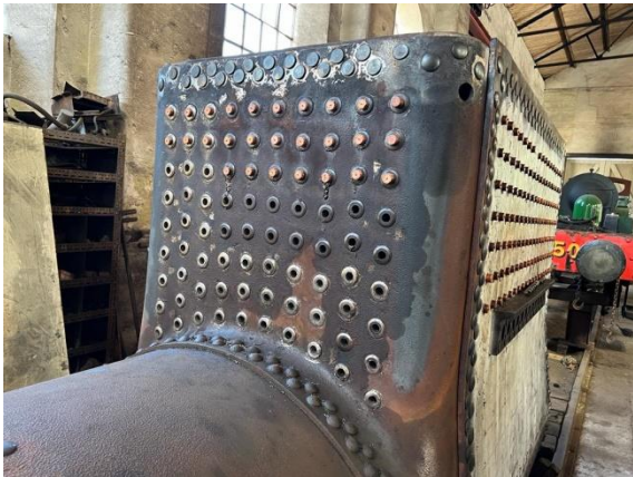
Copper stays also being added through the bushes on the throat plate.
